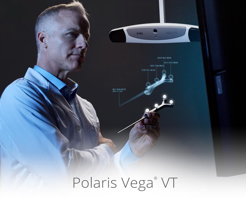
Envision new possibilities in OEM surgical tool tracking and navigation with the industry's first optical tracker to combine HD video and infrared (IR) tracking: the Polaris Vega® VT.
